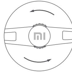
Turn the adjustment wheel counterclockwise to loosen the helmet.
